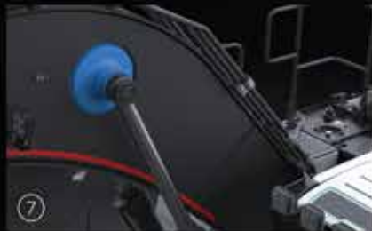
Reinforced boom cylinder cast bearing
